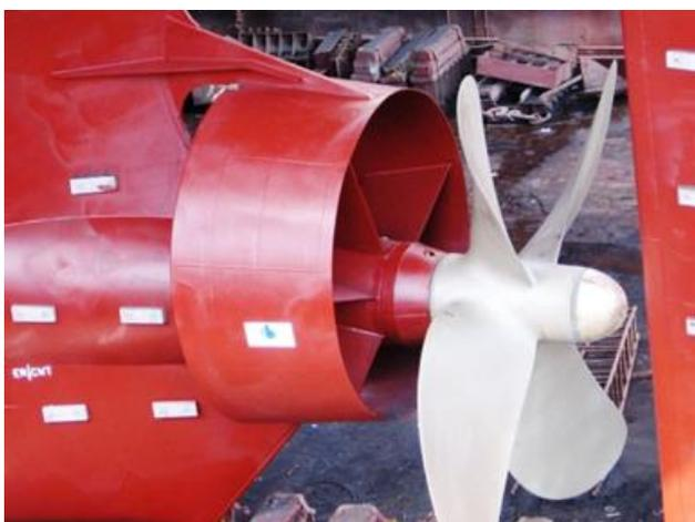
Figure 1 First Installed Full Scale Mewis Duct, STAR ISTIND, 54,000 tdw MPC, September 2009
